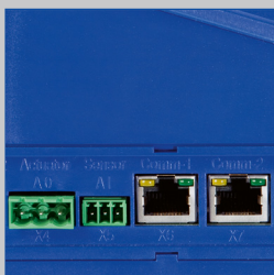
Plug sockets on the outside
