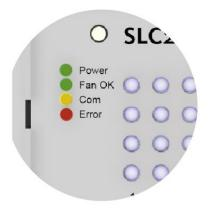
The unit has two damper position LEDs for each damper and an error LED. The fourth LED indicates the damper selected which can be tested directly via the unit. Press both buttons for T > 3 s to start an automatic search. As a result, SLC connections not being used will be deactivated and removed from the relay logic.
