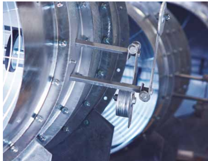
Axial fans with self-regulating closure flaps
