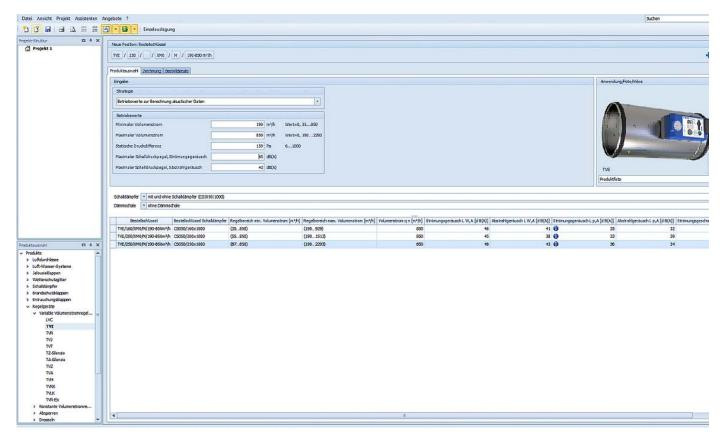
The Easy Product Finder allows you to size products using your project-specific data. Data on individually selectable operating points (e.g. volume flow rates, differential pressures and acoustics) can be calculated.
