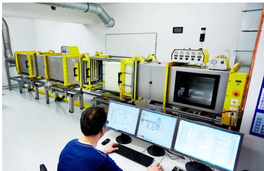
*The test rig for testing and classifying coarse dust and fine dust filters can now also be used for particulate filters.*
