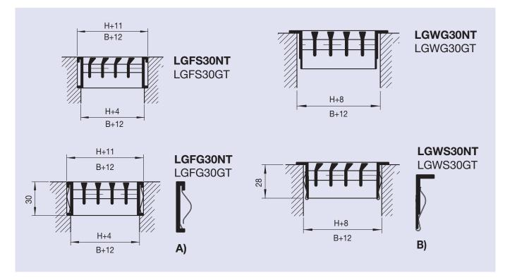
A) with spring clips KFF30, not suited for installation on ceiling
